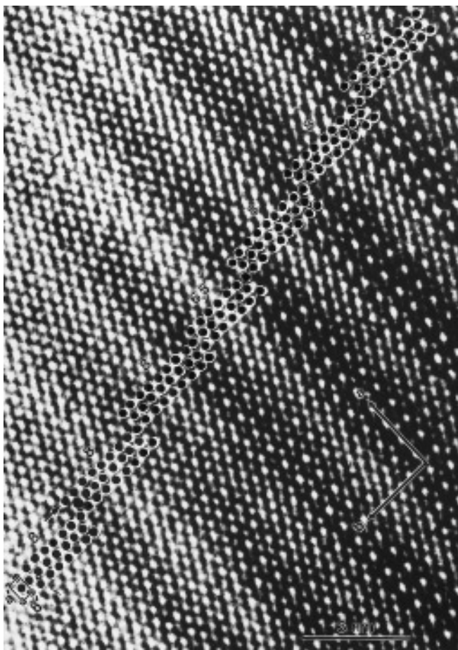
FIG. 2. An enlarged photograph of Fig. 1. The black dots giving rise to lattice fringes correspond to columns of metal atoms. Full circles represent approximate positions of the metal atoms and the rectangle with a' and b' corresponds an orthorhombic subcell. Lattice fringes have a modulation in their contrast. The contrast modulation has a sequence of 8, 8, 8, 6.5, 8, 8, and 8b' , which were determined from a variation of the spacing of the black dots shown in Fig. 3. The mean multiplicity of this crystal fragment is 7.7.
